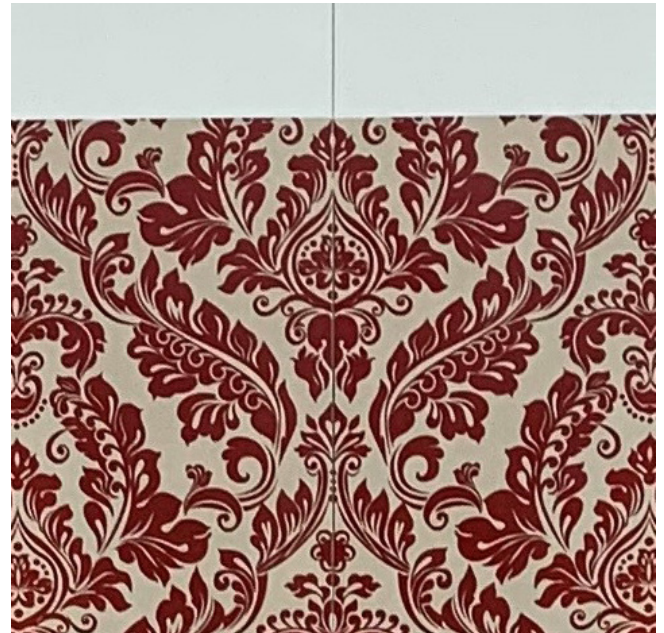
High resolution images showing dimensional and colour consistency of wallpaper panels from beginning of the roll – panel 1 (left side) to end of roll – panel 13 (right)
